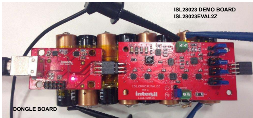
FIGURE 18. THE ISL28023 DEMO CONNECTED TO THE DONGLE BOARD AND A BATTERY PACK
